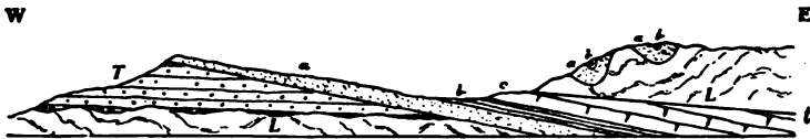
FIG. 996. — Diagrammatic section across the northwest Highlands of Scotland. L , Lewisian gneiss; T , Torridon sandstone; a , Arenaceous series of Cambrian; b , Middle series; c , Calcareous series; t , Thrust-plane. Note: The overthrusting is much more complex than is shown in this diagram. (From Lake and Rastall, Textbook of Geology .) (See also Fig. 550, p. 629, Pt. I.)
